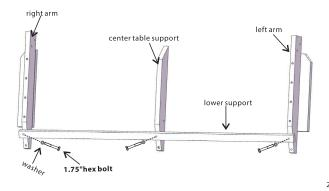
**[STEP 2]**: Use (2) 2.5" hex bolts, (4)washers, and (2) lock nuts to attach (2) outside verticals to left and right arm. Use(2) 3.5"hex bolts, (4)washers, and (2)lock nuts to attach table and middle vertical to center table support.
